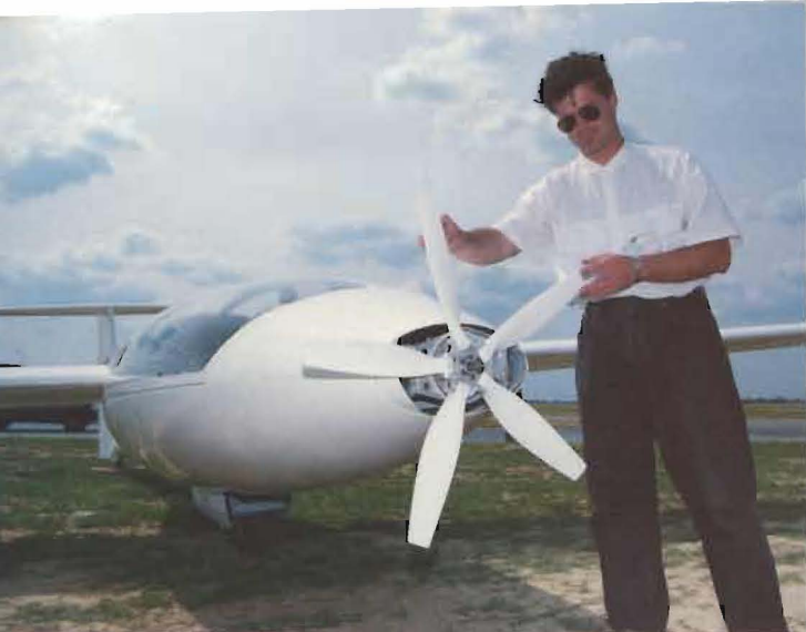
A two cylinder 32hp Rotax sustainer drives a five bladed folding prop in the Berlin Akafflieg B 13, which emerges forwards as the nose cone divides and retracts to either side.
